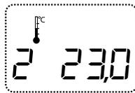
Display reading 3 shows the average temperature for the previous 24 hours
