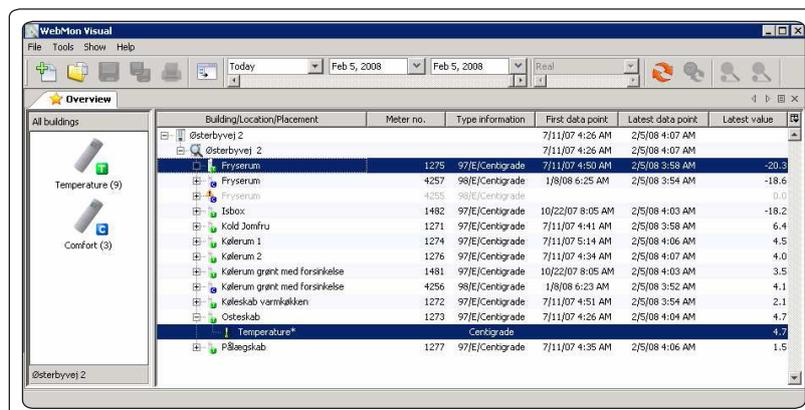
Example in which the meter no. 1275 (and its default registration) is selected as well as the temperature registration of meter no. 1273. After selection, you specify a period on the tool bar and click the "Create" button to create a new analysis with the selected registrations.
