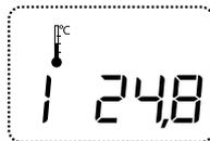
Display reading 2 shows the average temperature for the current 24 hours
