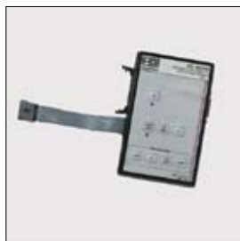
Fig 35: HG-SER 40 Service instrument
